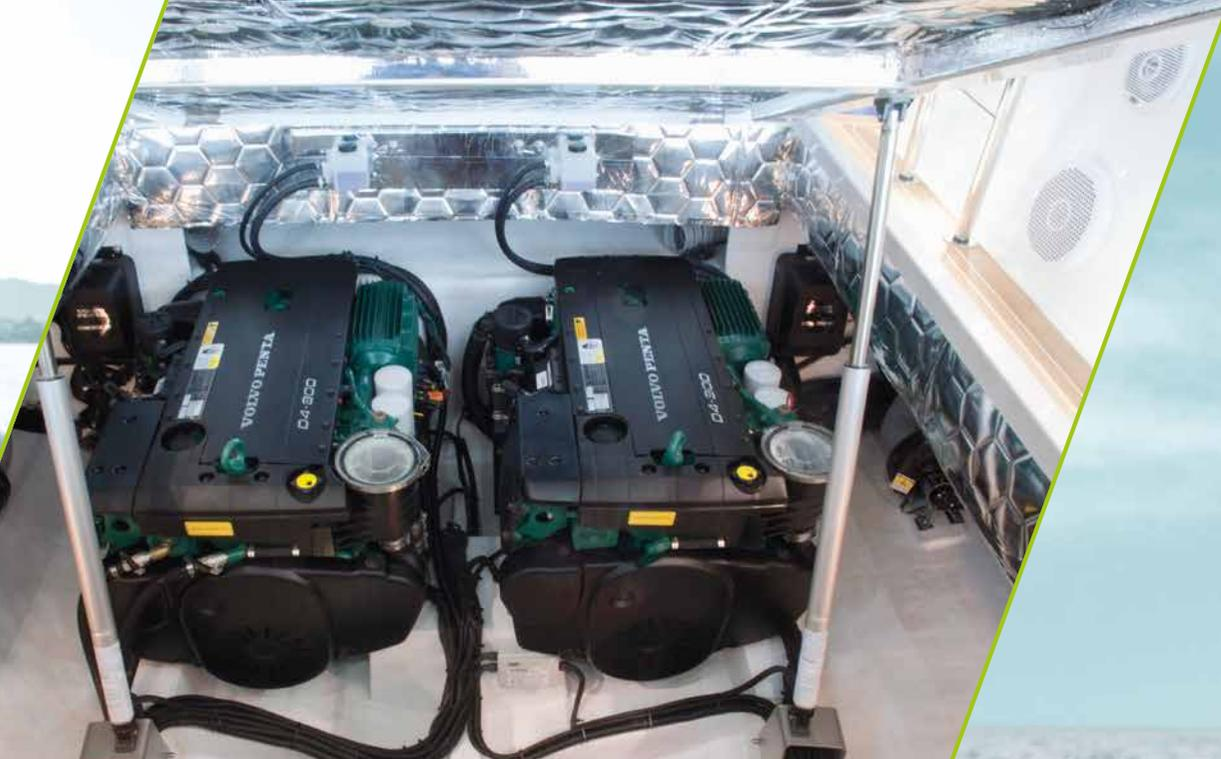
*power for propulsion: two Volvo diesel engines with 260 hp each*
