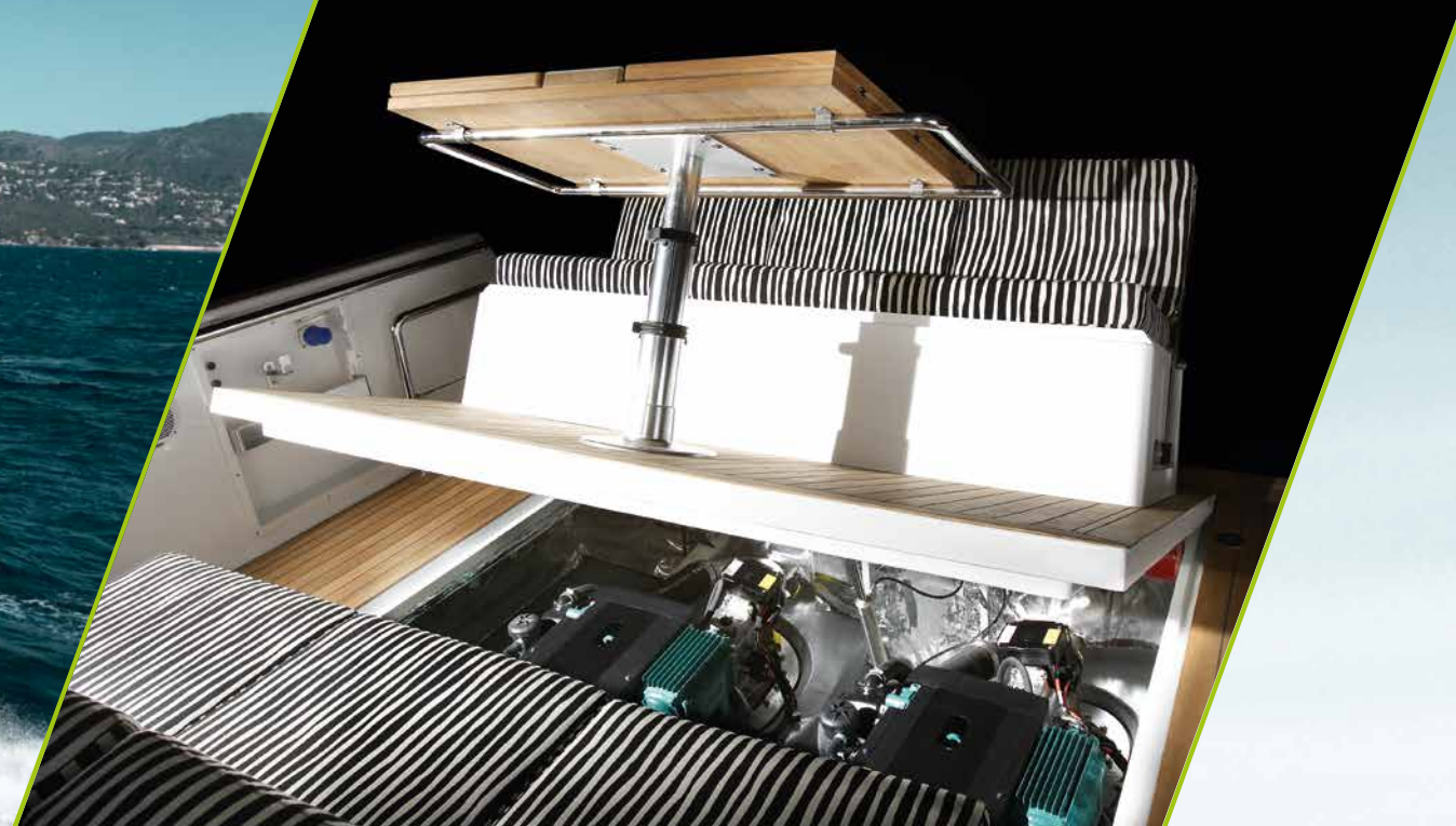
power for propulsion: two Volvo IPS engines with 370 hp or 435 hp
